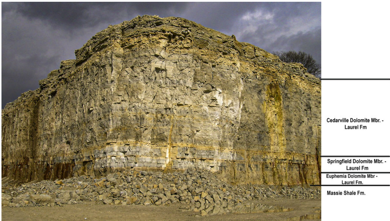
Figure 3. Exposed strata in highwall in the Pepcon Cement Quarry (see Fig. 1 for thicknesses).
