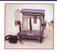
Anaesthesia Machine MP-3 This is a MP-2 with a ventilator, suction, and bag-in-a-bottle system added – a very sophisticated machine. The MP-3 also can be used as a "Drawover" machine similar to the MP-1 and MP-2.
