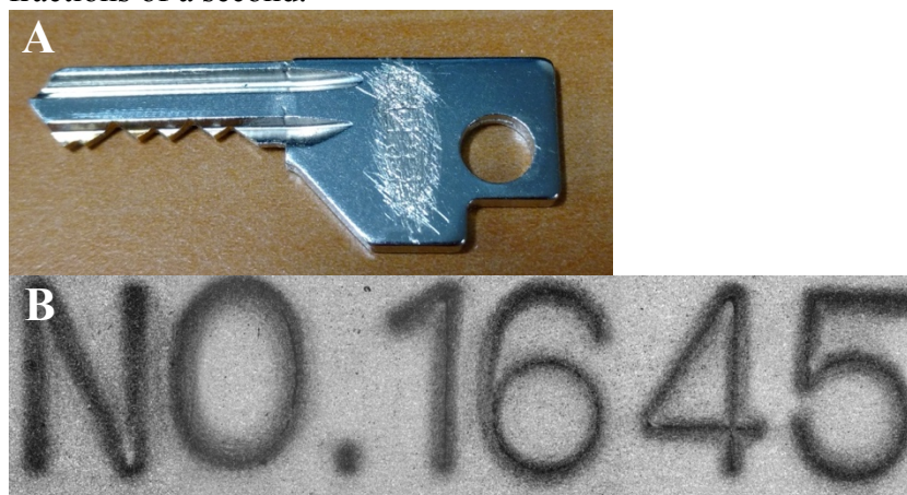
Figure 2. Reconstruction of a scratched off serial number with EBSD. The deformation induced by the imprinting of the serial number extends deeper into the metal of the key than is visible. As such, attempting to scratch it off does not remove all traces of the serial number and it can be recovered.
