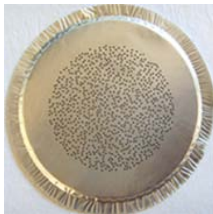
Figure 2 Loaded 47-mm foil impactor disk for PM 180–320 nm.
