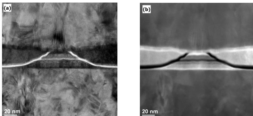
FIG. 1. (a) Bright-field TEM image of a commercial TMR reader, and (b) HAADF STEM image.
