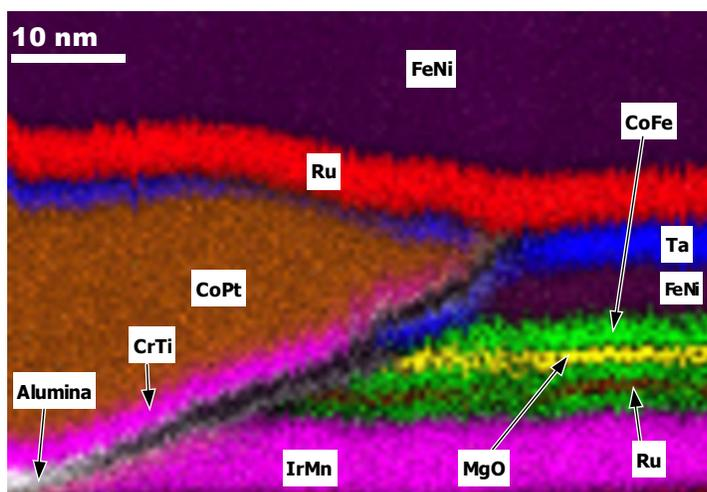
FIG. 3. Composite phase map reconstructed from the raw STEM/EDS dataset.
