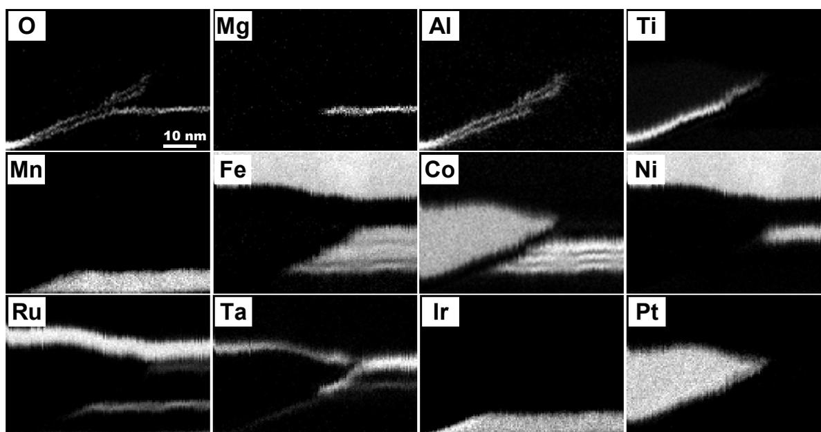
FIG. 2. Elemental maps reconstructed from the STEM/EDS dataset.
