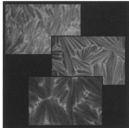
**ON THE COVER:** Optical micrographs taken between crossed polarizers of 2% hexanediol diacrylate polymerized (**top**) in the smectic C\* phase at 25°C, (**center**) in the smectic A phase at 50°C, and (**bottom**) in the isotropic phase at 70°C. For more information, see "Polymerization and Properties of Polymer-Stabilized Ferroelectric Liquid Crystals" by Christopher N. Bowman and C. Allan Guymon on p. 15 of this issue.
