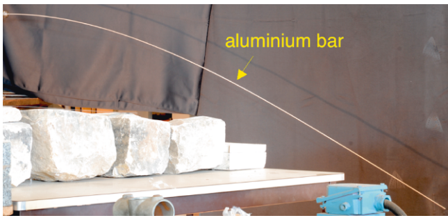
Fig. 12. (Color online) Aluminum bar bending under its own weight.
