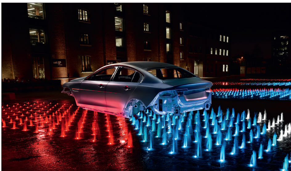
Innovate UK contributed around two-thirds of the £2 million cost of the REALCAR (REcycled ALuminum CAR) project, which enabled Jaguar Land Rover to make up to 50% of the bodywork of its new Jaguar XE from recycled aluminum. REALCAR brought together partners from industry and academia and led to the development of a new aluminum alloy that reduces the weight of a car. Credit: Jaguar Land Rover.
