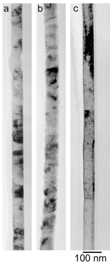
FIG. 2: Cross-sectional TEM images of: (a) the Fe film annealed in vacuum at 700 K for 60 min., (b) the Fe film surface in (a), after exposure to nitrogen (0.75 Pa) at 673 K and cooling to 300 K, (c) the Fe film surface in (b), after the heating cycle in the TDMS process from 300 K up to 950 K. The thickness of the films is: 54 \pm 2 nm (a), 68 \pm 6 nm (b), 55 \pm 2 nm (c).
