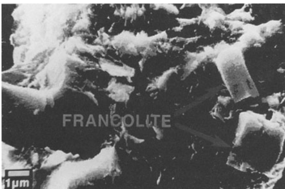
Figure 4. Crystallites of francolite in kaolinite matrix. Flint clay from Landwehr No. 1 pit, Gasconade County, Missouri.
