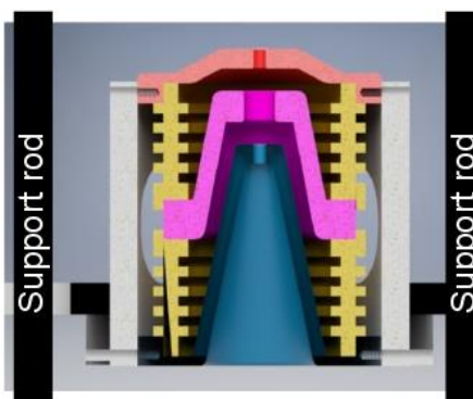
Fig 2. NanoMi Einzel lens. Biased electrode (pink) is placed between two grounded electrodes (blue and red) separated by an insulator (yellow). The entire assembly is placed inside a stainless steel puck with mounts (gray). The column can be composed either of identical lens or various optical elements mounted on support rods (black). The stainless steel puck is about 50 mm tall and about 50 mm diameter.
