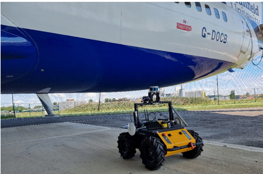
Figure 18. The Clearpath's Husky navigating inside the DARTeC's smart hangar.
