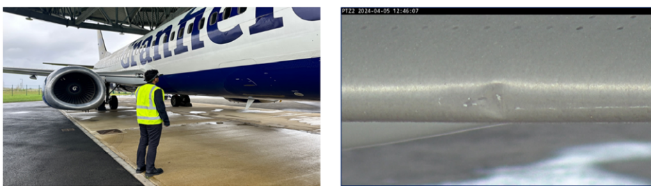
Figure 14. (left picture) An MRO inspector is wearing the hands-free device and performing the IA check (right picture). The dent is captured from the PTZ fixed camera that is fixed in the DARTeC smart hangar.
