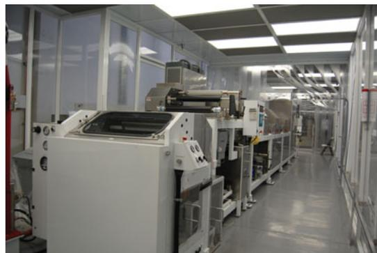
Solarmer's roll-to-roll pilot production line for the manufacture of organic photovoltaic modules.
