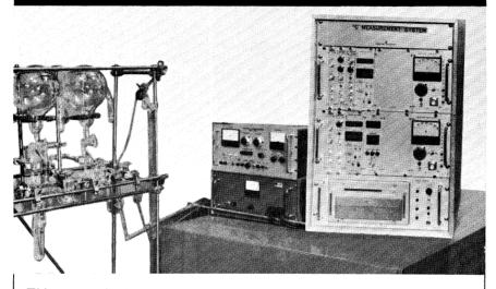
This system is designed to measure efficiently the value of radioactivity emitted from <sup>14</sup>C included in a sample by means of Multi-anode anti-coincidence gas proportional counter.
