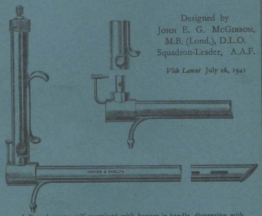
A Bronchoscope self contained with battery in handle, dispensing with entangling cables.
