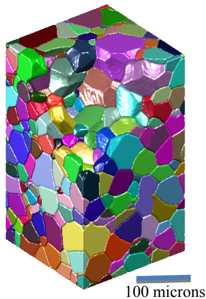
FIG. 2. Example of visualization of the grain structure of a Timet \beta 21s titanium alloy (the colors in the figure are random). The data is acquired using phase contrast tomography at the ID19 beam line at the European Synchrotron Radiation Facility, Grenoble, France.
