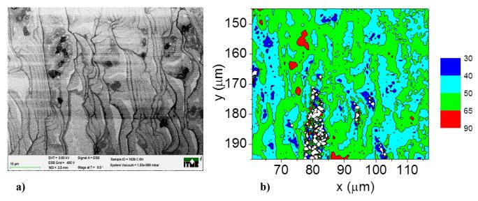
**Figure** 2. SEM images recorded in dual-channel mode, showing the contrast in the stack of graphene layers grown on C-terminated SiC-6H; a) SE1 image, b) low-loss BSE image; areas of random misorientation are brighter in SE1 image and darker in BSE image.
