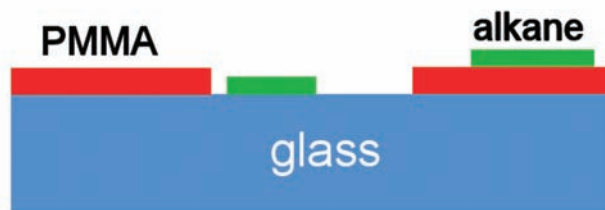
Fig. 3: Schematic of the glass-PMMA-alkane sample, 7.1 nm PMMA film and 4.2 nm alkane film on glass.
