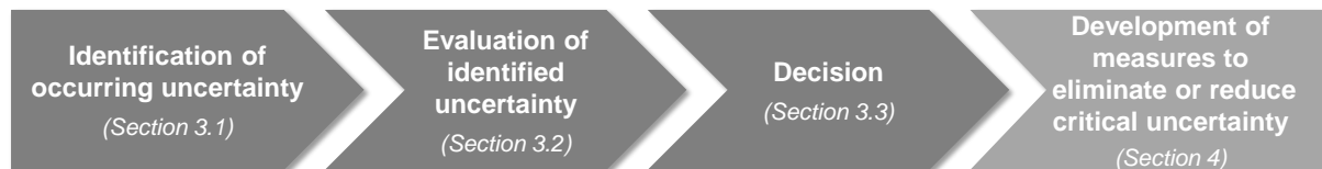
Figure 3. Structure of the uncertainty analysis (cf. Vorwerk-Handing et al., 2020b , based on Engelhardt et al., 2009 )
