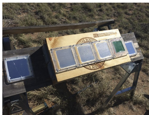
Figure 5. EDS film with reflective electrodes on field test site.
