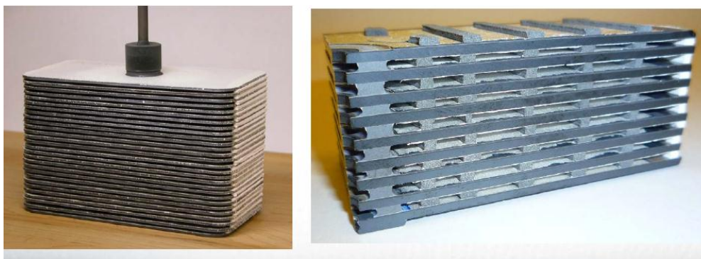
Figure 2. Photos of the cell stack, and a cut section of a cell stack (note glass seal in section view)
