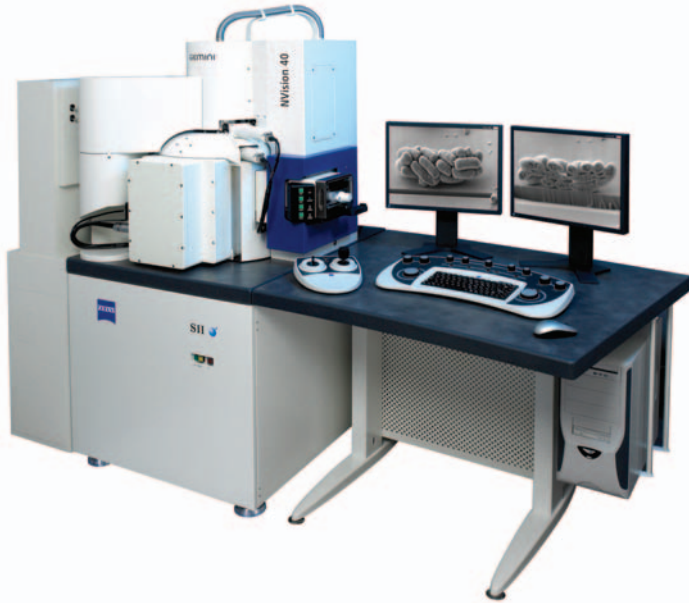
Fig 2.: The NVision 40 CrossBeam® Workstation. The system is comprised of the Gemini® SEM column, an ion column with accelerating objective lens technology, and a mass flow controlled multi channel GIS. The ion column is located at a 54° angle from the SEM column. The system is also equipped with in-lens SE and BSE detectors, a chamber SE detector, and two infrared chamber scopes. There are additional ports for STEM, 4QBSE, EDS, and EBSD detectors as well as sample manipulation tools.
