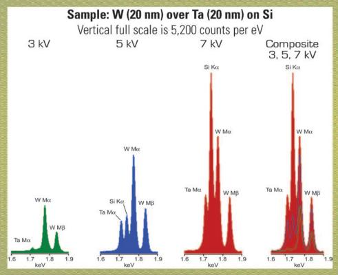
Microcalorimeter spectra for a W (20 nm) over Ta (20nm) bilayer on a Si substrate is shown at left. The MICA-1600 clearly resolves the Ta, Si and W peaks around 1.75 keV and enables surface analysis of nanometer-scale films. The spectra also illustrate how the depth of the X-ray excitation volume increases with increasing beam voltage.
