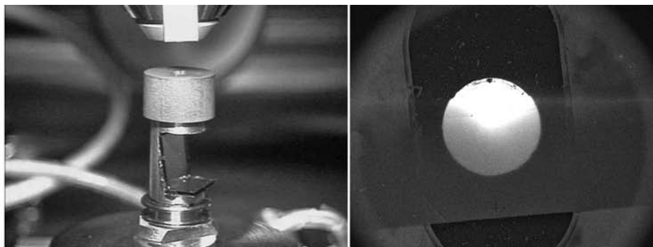
Figure 3, left: Design for a “STEM-in-SEM” sample holder. The overall height is 2.5 cm.
