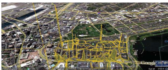
Figure 1: Methane leaks from natural gas pipelines in the Beacon Hill neighborhood of Boston. Yellow bars represent methane concentrations in parts per million; the highest values recorded exceed 15 times background levels.
