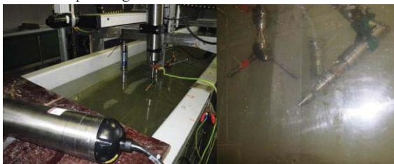
Figure 1: The flume Eddy Covariance deployment (Sept. 2011) showing sensor set-up (velocimeter, left and microelectrode, right).
