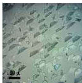
Figure 2: The reacted calcite surface imaged within the X-ray beam footprint, observed under reflected light microscopy. Cerussite occurs as trapezoidal precipitates showing euhedral (021) growth face.
