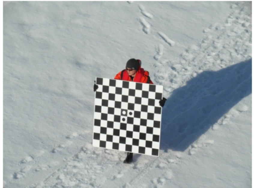
Fig. 3. Calibrating the system at an ice station using a checkerboard calibration pattern.
