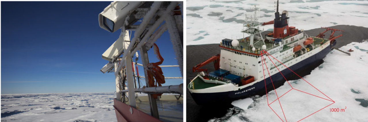
Fig. 1. The Polar Sea Ice Topography REconstruction System, and its approximate viewing area.
