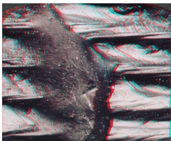
Fig 4 Between-Belt Tearing Lip
