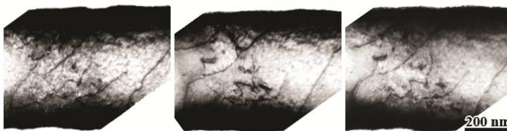
FIG 3. Aligned bright-field TEM images of 16% pre-strained Mo fiber from a tilt series taken every 2^\circ over a range of 57^\circ . Example images are tilted \pm 18^\circ about 0.6^\circ .
