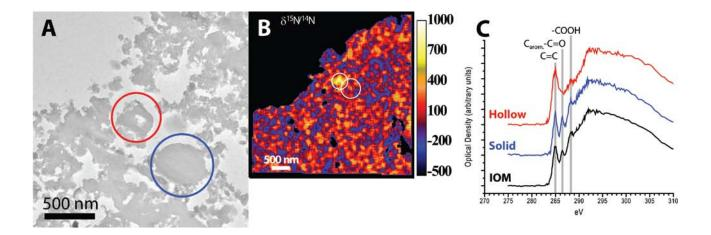
**Figure 1.** Correlated (A) TEM, (B) SIMS, and (C) XANES characterization of a hollow (red circle) and a solid (blue circle) nanoglobule compared with surrounding insoluble organic matter (IOM) from the meteorite EET92042.
