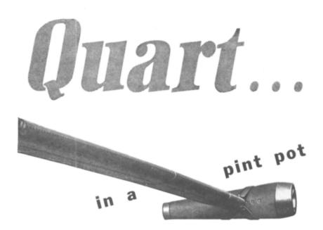
Less than four feet in length, the pint-sized Saunders-Roe pulse jet engine packs a barrel-load of power Developed by the Saunders-Roe Helicopter Division, it is one of the simplest forms of power unit and, fixed to the tip of each helicopter rotor blade, provides a torque-free drive with a high overall power-to-weight ratio, virtually eliminates the heavy and costly transmission shafting and gearing and makes possible a greatly simplified and lighter airframe
