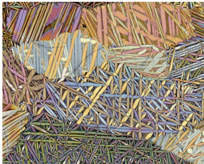
**People's Choice Award.** Carbon-free martensite, formed by casting a CoFeSi alloy into a copper mold. Several generations of martensite needles are clearly distinguishable, and the former austenite grains can be identified. Metallographic specimen etched with color etching agent V2A-Beize and imaged in reflected light microscope. Image by Felix Trauter, Materials Research Institute, Aalen University, Aalen, Germany.
