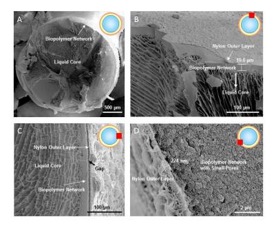
**Figure 1.** Fig. 1. (A) Low magnification image of multilayered capsule, (B) Close-up view of the multilayered capsule (red region) showing the liquid core, biopolymer shell and, the thin nylon outer layer along with the thickness of the biopolymer network, (C) Close-up view of the capsule showing the gap between the layers and, (D) SEM image showing the thickness of the outer nylon layer and porous biopolymer network.
