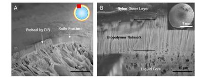
**Figure 2.** Fig. 2. (A) SEM image showing the strong curtain effect of FIB milled surface and, (B) SEM image showing the three different regions of the multilayered capsule using cryo-FIB technique along with the intact capsule (on the top right) which was milled using FIB.
