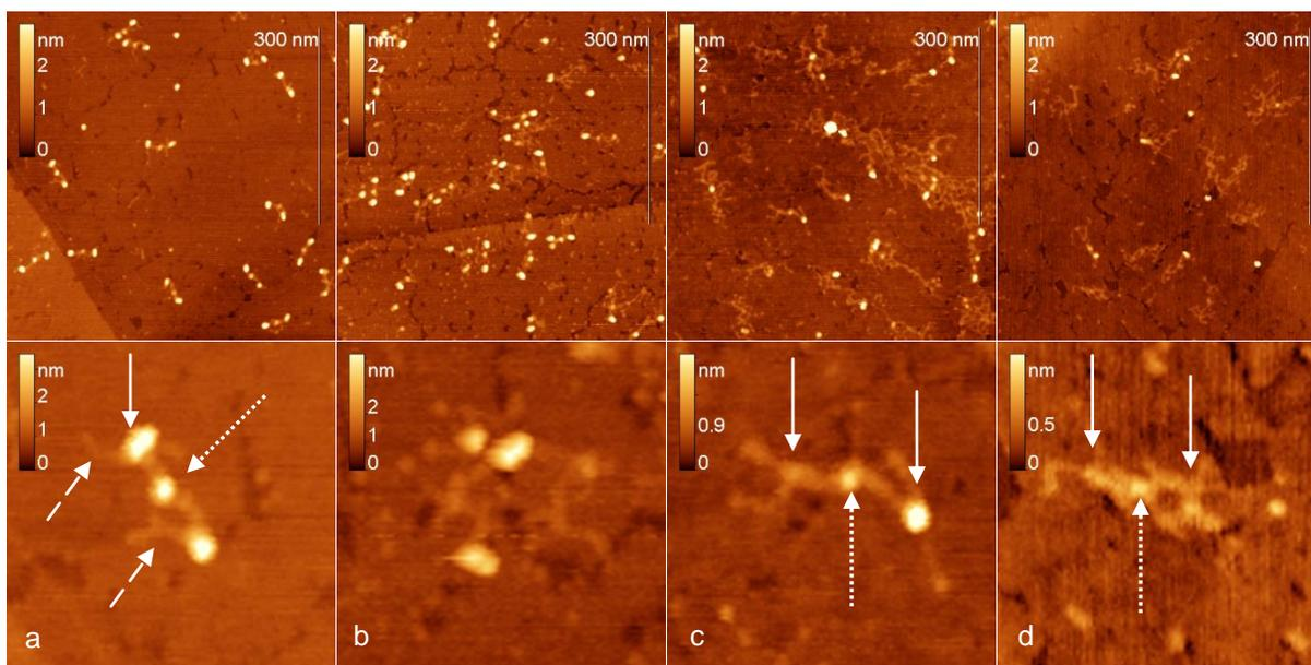
**Figure 1.** AFM images of fibrinogen molecules adsorbed on GM-HOPG surface for (a) 10 sec, (b) 1 min, (c) 3 min, (d) 10 min. Bottom row represents enlarged regions ( $100 \times 100 \text{ nm}^2$ ) from the corresponding AFM images on top ( $500 \times 500 \text{ nm}^2$ ).
