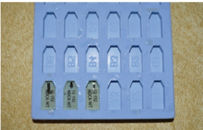
Figure 8: Polycarbonate filter curled in propylene oxide (top). Curled filter cut into pieces and embedded (bottom).
