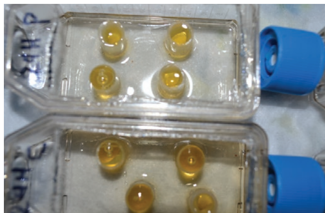
Figure 3: Embedding tubes filled with resin on the second day.
