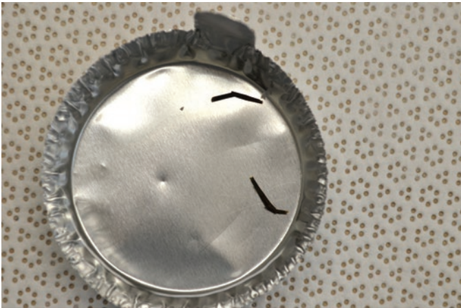
Figure 7: Polycarbonate filter separated from its holder after osmium post-fixation.
