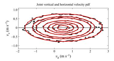
Figure 2. Joint density of  $v_h$ ,  $v_v$ , horizontal and vertical particle velocities at local maxima from (B1) (smooth, red curves) together with empirical p.d.f. from 100 000 simulated Slepian realisations (wiggly black curves). Level curves as in figure 1. The wave spectrum is J20 at infinite depth. The level curves enclose 10:20:90,95, 99% of the distribution.
