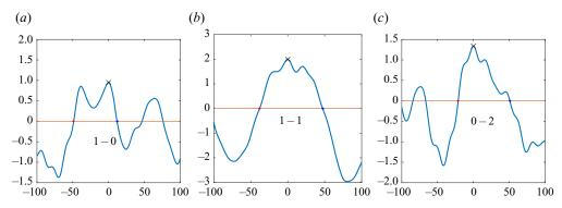
Figure 8. Illustration of the discrete dependence of crest location (marked with  $\times$ ) and the number of local maxima in a crest period. The code *x*–*y* indicates the number of local maxima to the left and right of the crest, respectively.
