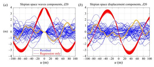
Figure 4. Slepian wave and displacement components for models in figure 3 plotted separately.
