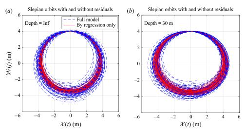
Figure 5. Orbits for the top particles in figure 3 according to models (5.13). (a) Infinite depth; (b) depth 30 m. Red curves are the symmetric regression orbits, blue dashed asymmetric curves include the residuals. The Airy orbital eccentricity of surface particles at water depth h = 30 m is  $\cosh(k_p h) / \sinh(k_p h) = 1.14$  for this narrow spectrum with peak frequency  $\omega_p = 0.046$  rad s<sup>-1</sup>. The observed average eccentricity of the simulated regression orbits is 1.12.
