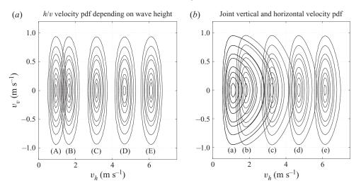
Figure 1. Joint horizontal/vertical velocity depending on wave height for a J20 spectrum. (*a*) At wave max equal to  $w_0$ . (*b*) At wave max exceeding  $w_0$ . (A/a)–(E/e):  $w_0 = [0.25 \ 0.5 \ 1 \ 1.5 \ 2] \times H_s$ . The level curves enclose 10:20:90, 95, 99, 99.9% of the distribution.
