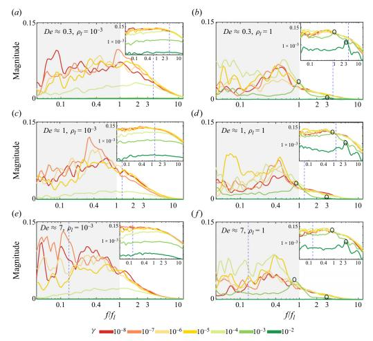
Figure 5. Frequency distribution of the fibres from the wavelet analysis, for  $De \approx 0.3, 1, 7$ , for (a,c,e) neutrally buoyant fibres  $(\rho_l = 10^{-3})$  and (b,d,f) denser-than-fluid fibres  $(\rho_l = 1)$ .
