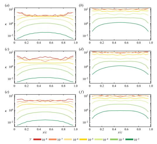
Figure 8. The curvature  $\kappa$  plotted as a function of the normalised length s/c, along the fibre length at (a,b)  $De \approx 0.3$ , (c,d)  $De \approx 1$ , and (e,f)  $De \approx 7$ , for (a,c,e) neutrally buoyant and (b,d,f) denser cases.
