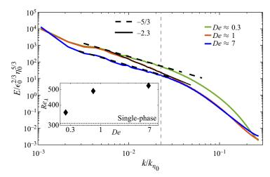
Figure 2. Energy spectra of the turbulent polymeric flows at different Deborah numbers De. The vertical dashed line represents the wavenumber corresponding to the fibre length. The inset shows the resulting Taylor Reynolds number  $Re_{\lambda}$  for each of the cases.
