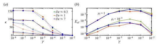
Figure 7. (a) Curvature and (b) elastic energy stored by the neutrally buoyant and denser fibres at various *De*. Open and closed symbols are used to distinguish neutrally buoyant and denser cases, respectively, while in (a), we use dotted and solid lines to distinguish the maximum and mean curvatures.
