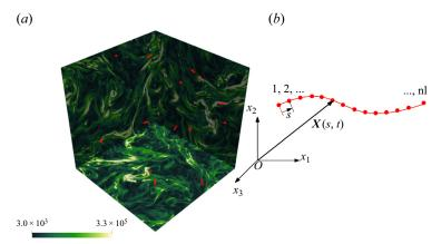
Figure 1. (a) A qualitative snapshot from the DNS simulations for  $Re_{\lambda_0} \approx 310$  and Deborah number  $De \approx 7$ , where fibres of various rigidities are dispersed in a tri-periodic domain. The three back planes are coloured based on the trace of the polymer conformation tensor, and the red lines represent the fibres. (b) Schematic of the fibre and the Lagrangian points.
