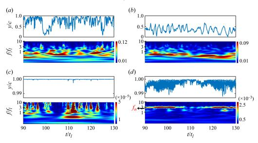
Figure 4. Time histories and wavelet transform of the fibre end-to-end displacement at the smallest Deborah number  $De \approx 0.3$  for fibres that are (a) neutrally buoyant, flexible ( $\rho_l = 10^{-3}$ ,  $\gamma = 10^{-8}$ ), (b) denser-than-fluid, flexible ( $\rho_l = 1$ ,  $\gamma = 10^{-8}$ ), (c) neutrally buoyant, rigid ( $\rho_l = 10^{-3}$ ,  $\gamma = 10^{-2}$ ), (d) denser-than-fluid, rigid ( $\rho_l = 1$ ,  $\gamma = 10^{-2}$ ).
