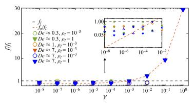
Figure 6. The flapping frequency of the fibre from a Fourier analysis, as a function of the bending rigidity  $\gamma$ . The inset reports a zoomed view of the same plot in a log-log scale. For dense fibres, we include results from additional simulation with  $\gamma = 10^{-1}$  and 1.
