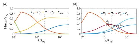
Figure 3. (a) Flux contributions from (3.1) (normalised with the turbulent energy dissipation rate) plotted with respect to the wavenumber k, at  $De \approx 1$ . (b) The variation of the nonlinear energy flux  $\Pi_f$ , fluid dissipation  $D_f$ , polymer flux  $\Pi_p$  and polymeric dissipation  $D_p$ . The vertical dashed lines represent the wavenumber corresponding to the fibre length.
