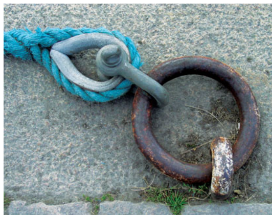
To combat the effects of materials degradation, this mooring ring, shackle, and thimble with rope uses three different techniques. The ring and eye bolt was originally painted, the shackle and thimble has been galvanized (zinc coated), and the mooring line was made of nylon. Courtesy of Erik Svedberg.
