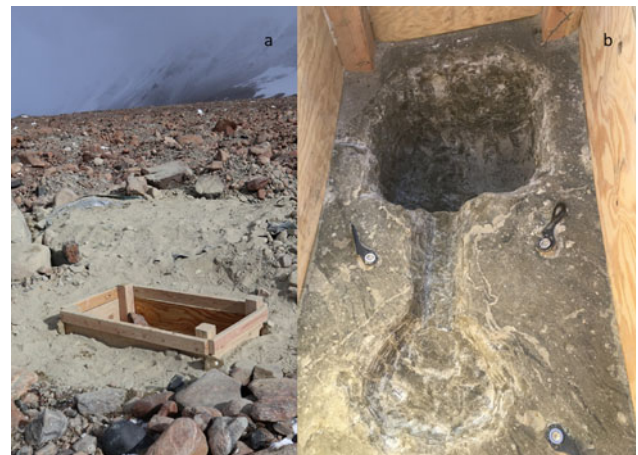
Fig. 7. (a) At the Ong Valley drill sites a layer of sediment was covering the ice surface. Once the ice was exposed, a timber barrier was built to support the drill rig and prevent loose sediment from falling into the borehole. (b) A channel was carved into the marbled ice to direct the drill fluid to a sump where it could be pumped into the filter tank. The borehole was drilled into the center of the bowl at the bottom of the image.
