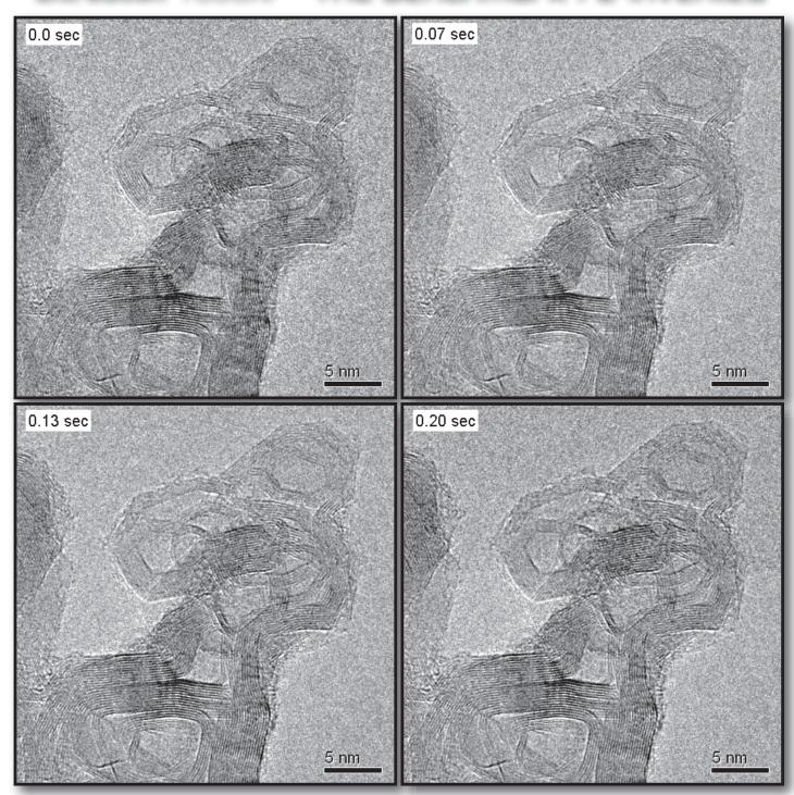
Individual frames of a captured digital streaming video sequence of graphitized carbon sample with Gatan UltraScan®1000XP CCD camera on a 200 kV TEM. The camera was operated at 16 fps. TEM magnification = 400 kx.
