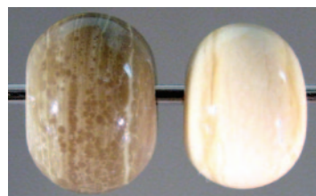
Figure 3: Beads made from Effetre 264 Ivory glass. The left bead was produced in a neutral flame and then exposed to the torch plume from a melted gather of Effetre 456 glass. It turned silvery gray as compared to the normal color of this glass when melted in a neutral flame with no exposure.
