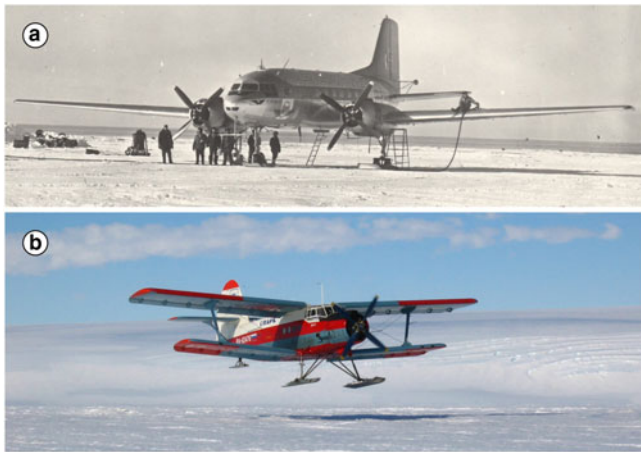
Fig. 4. Russian short-range Ilyushin Aircraft IL-14 (a), the main airline used in 1960s–1980s for airborne geophysical investigations and short-range Antonov Aircraft An-2 (b), which has been used since 1989 (photo from PMGE archive).
