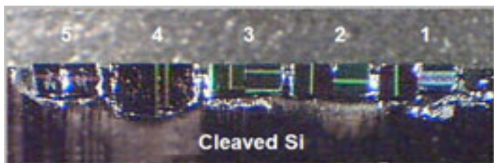
Using the Centar's 3D EAC™ (Exact Angle Control), the Si carrier is aligned and side 1 of all the specimens is polished to the same plane.
