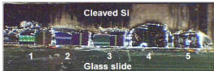
The row of specimens is then super-glued to a glass slide. After the glue has cured, the Si carrier is removed by melting the wax away. This transfers the specimens to the glass slide. Shown schematically below
