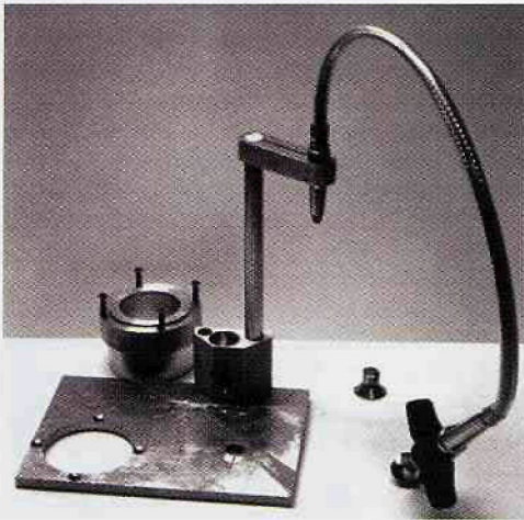
Figure 1: Microscope mounting bracket and eyepiece bushing for a Nikon Coolpix camera.
