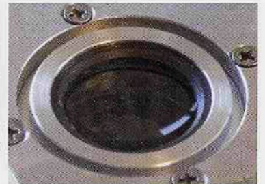
Figure 5: Close-up view showing the recess for the Coolpix camera lens flange to minimize the eyepiece to lens gap.
