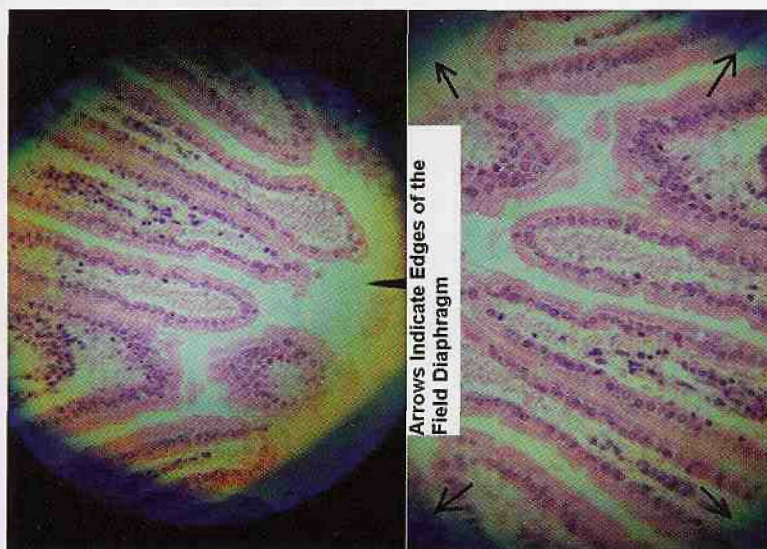
Figure 6: Coolpix camera lens zoomed out to show the full field of view of the microscope with the field diaphragm set to be just visible at the edge of the field of the 18 mm field number of the binocular viewing eyepieces
