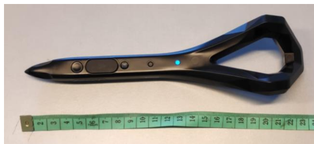
Figure 4. Logitech VR ink Pilot Edition (“Logitech VR Ink Pilot Edition - Ink Differently”, n.d.). Contains two force sensitive controls (index finger and stylus tip), clickable 2D touch strip and dual sided grip grab buttons. 232x64x42mm, Weight 68g
