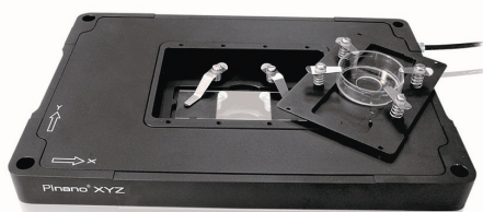
XYZ flexure stage, <1nm resolution
