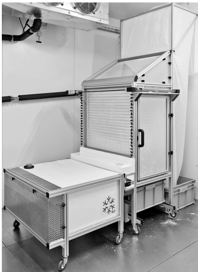
Fig. 3. Snowmaker in operation in the cold laboratory.
