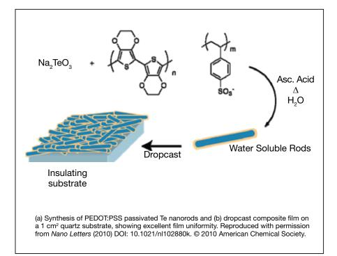
(~400 μV/K), but relatively low electrical conductivity and high thermal conductivity. The research team has shown that Te nanorods can be synthesized *in situ* into a highly electrically conductive, thermally insulating polymer (PEDOT: PSS,  $\sigma$  >100 S/cm,  $\kappa$  ~ 0.2W/m² K) in a water solution (see figure).
