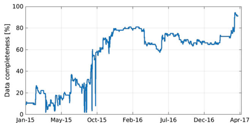
Fig. 3. Temporal development of data completeness for the G-network (Fig. 1A). 100% completeness corresponds to continuous data being available from all 69 \times 5 sensors.
