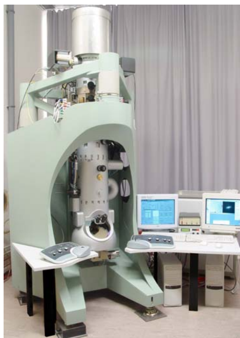
Fig. 2. Photograph of the UHR-TEM with the column suspended in the support structure.
