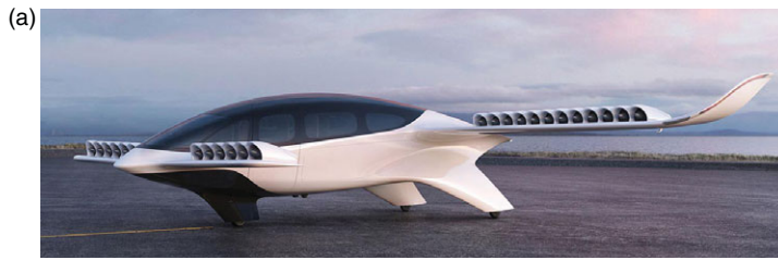
(a) An eVTOL aircraft with vectored thrust distributed propulsion system, Lilium
